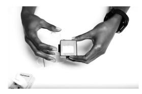
You must keep the device charged using any method that is most suitable. To charge device while attached to your hand using the portable charger, simply place the portable charger on top of the device being sure to make contact with the side of the watch and be sure to look for the green indicator light as pictured.
